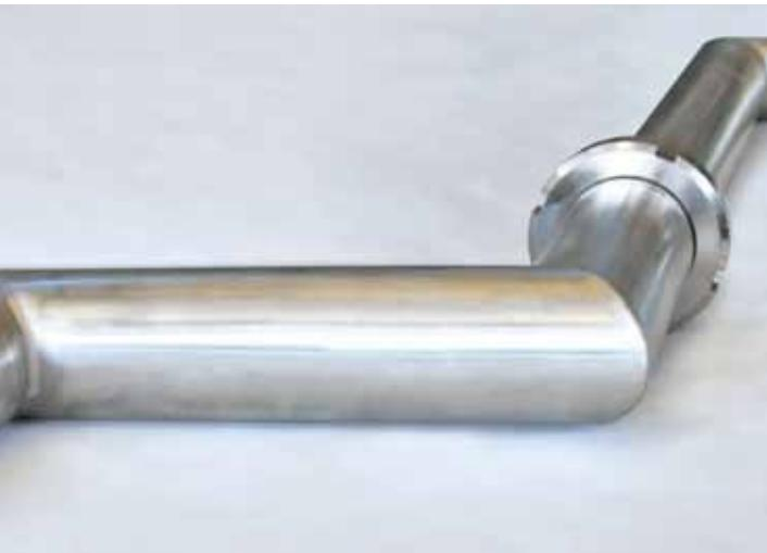
Thanks to their special technology and high insulation power, CTLs are the safest and most effective means to transfer cryogenic fluids. The lines consist of an inner pipe or hose equipped with multi-layer insulation, and an outer pipe or hose with a vacuum cavity. Vacuum ensures heat convection process insulation whereas radiation is prevented by the multi-layer insulation of the inner pipe, supported by spacers having a very low coefficient of thermal conductivity.
